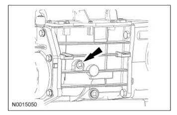
5. NOTE: Do not overfill the transmission. This will cause transmission fluid to be forced out of the case.
